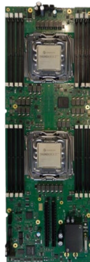
Mont-Blanc 3 prototype blade, equipped with Cavium ThunderX2 ArmV8 processors
